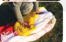
**Step 5.** Strap the Folding Pillow below the LE - at the point of the first fold. The pillow reduces the angle of the fold and helps preserve the plastics. Next fold the TE over the LE being careful to not fold with tight angles.
